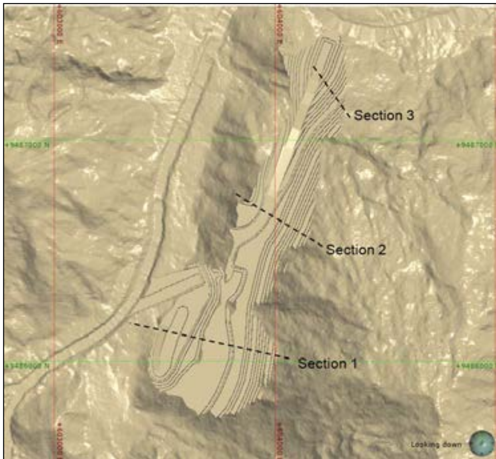
Figure 10-25: Plan view showing positions of analysis sections relative to the initial quarry and spillway design
