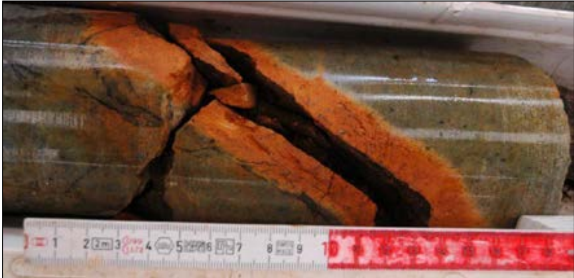
Figure 3-8: An example of intense weathering in wall rock of upper dunite bedrock
