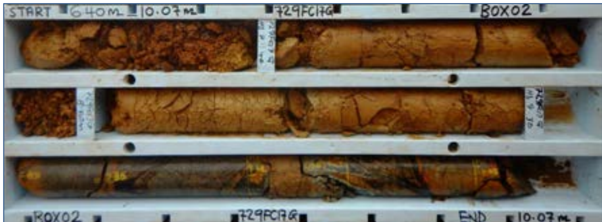
Figure 3-30: Core photograph showing soil-like overburden material immediately above highly fractured rock in drill hole LH7 (6.4–10 m)
