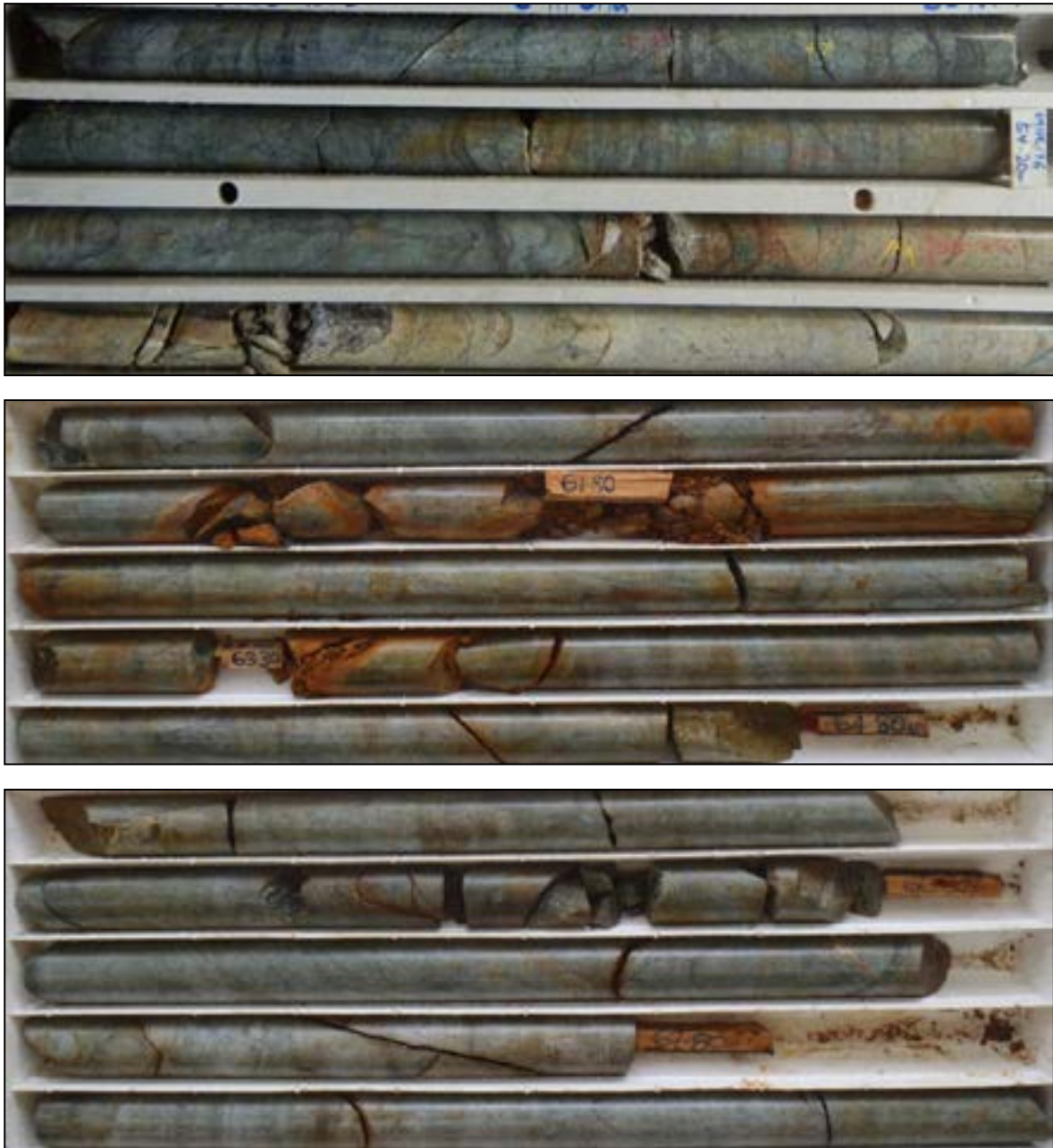
Figure 3-95: Examples of drill core from the northern part of the quarry
