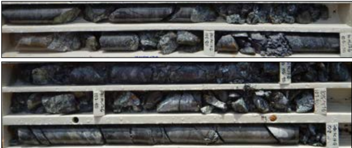
Figure 3-72: Core photographs of possible intersection in the south quarry area in hole Q6
