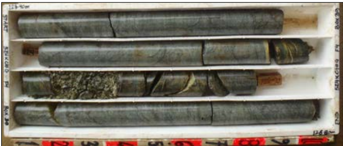
Figure 3-12: A small (fourth order) fault with gouge in good quality dunite
