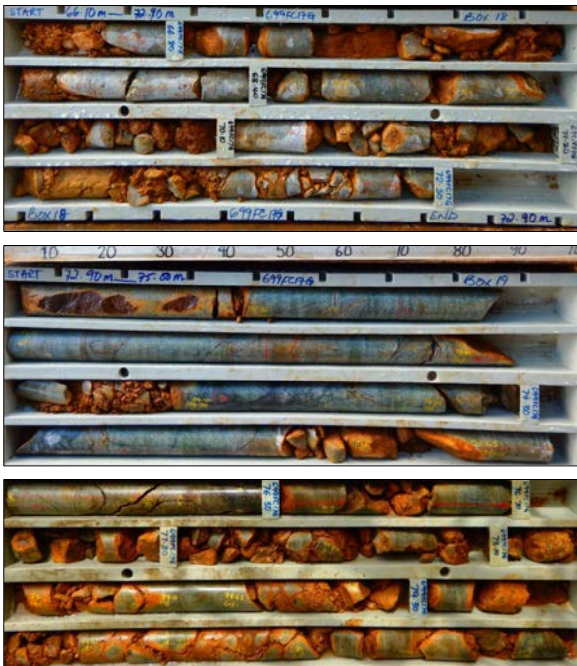
Figure 3-27: Core photograph showing variability of zones of highly fractured and oxidised rock with deteriorating matrix and/or soil-like infill in drill hole LH3 (66–80 m)
