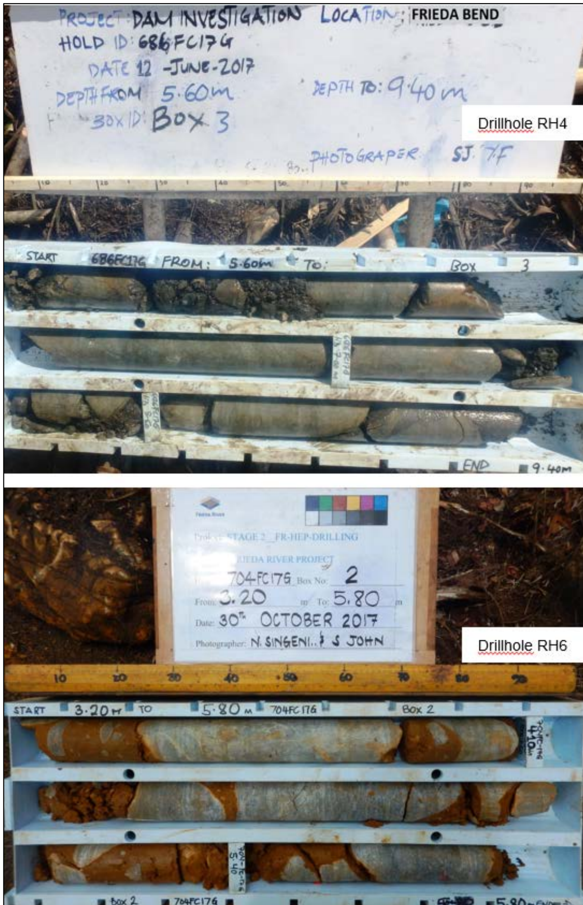
Figure 8-3: Core photos from holes RH4 and RH6 – Frieda River riverbed representative of foundation level (~5 m)
