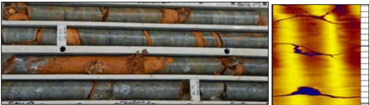
Figure 3-33: Slightly weathered to unweathered bedrock with joint infills of variable thickness (left), shown in acoustic televiwer survey image (right)
