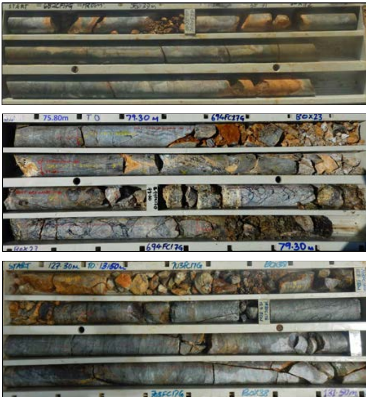
Figure 3-68: Core photos illustrating the nature and variability of conditions along Fault 2 in the right abutment: (above) very thin gouge zone with oxidisation of surrounding joints in hole RH1; (middle) oxidised fracture zone with localised gouge in hole SW5; and (bottom) fractured, oxidised zone in hole SW6
