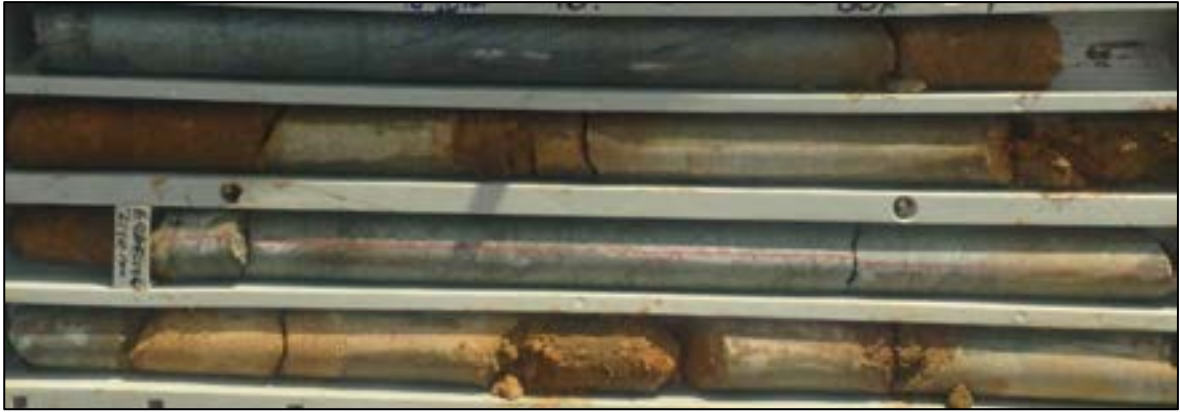
Figure 3-32: Moderately to slightly weathered bedrock with thick joint infills
