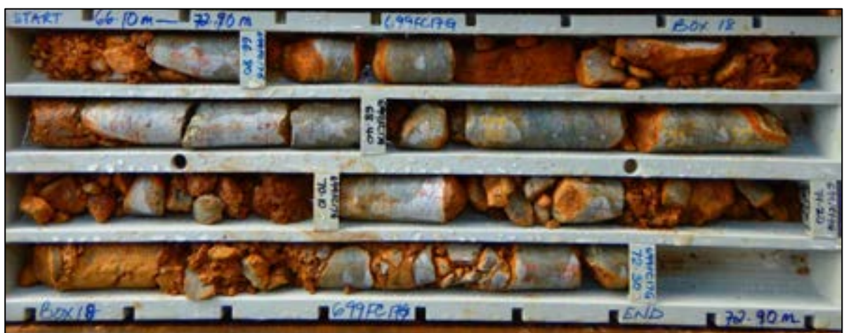
Figure 11-11: Core photograph showing soil-like overburden material immediately above highly fractured rock in drillhole LH7, from 6.4 m to 10 m depth
