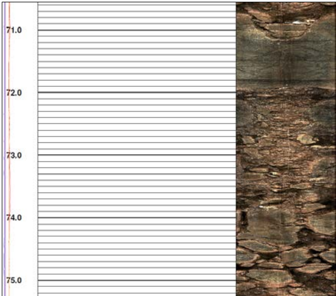
Figure 3-28: Downhole OTV image in drill hole LH7 showing potential landslide materials below 70 m depth downhole
