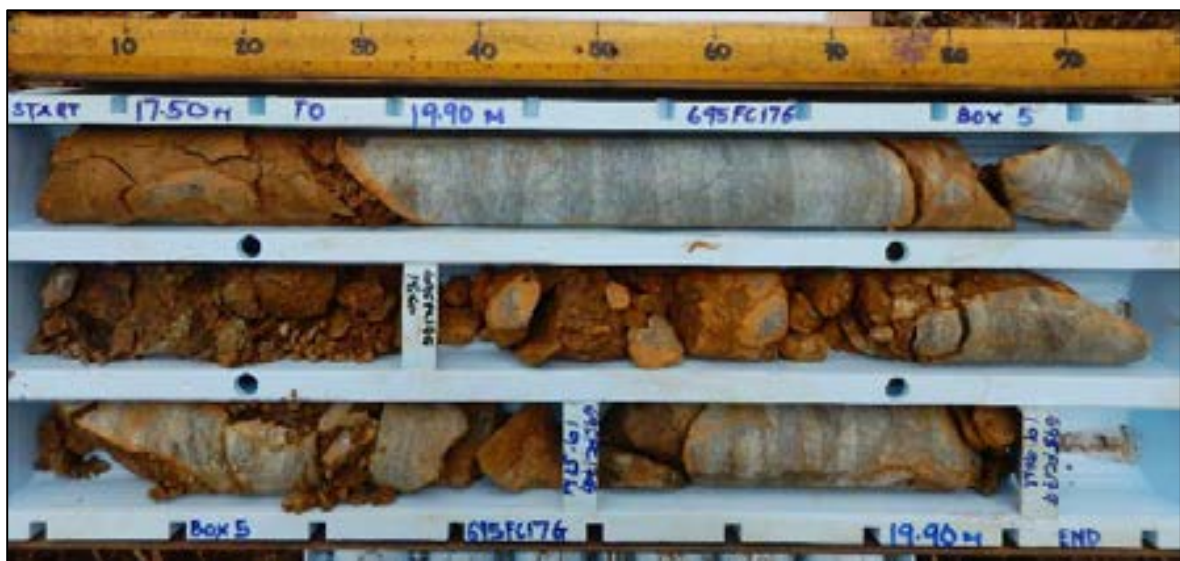
Figure 3-31: Drill hole SW4 showing boulder overburden material over the bedrock (17.5–19.9 m)
