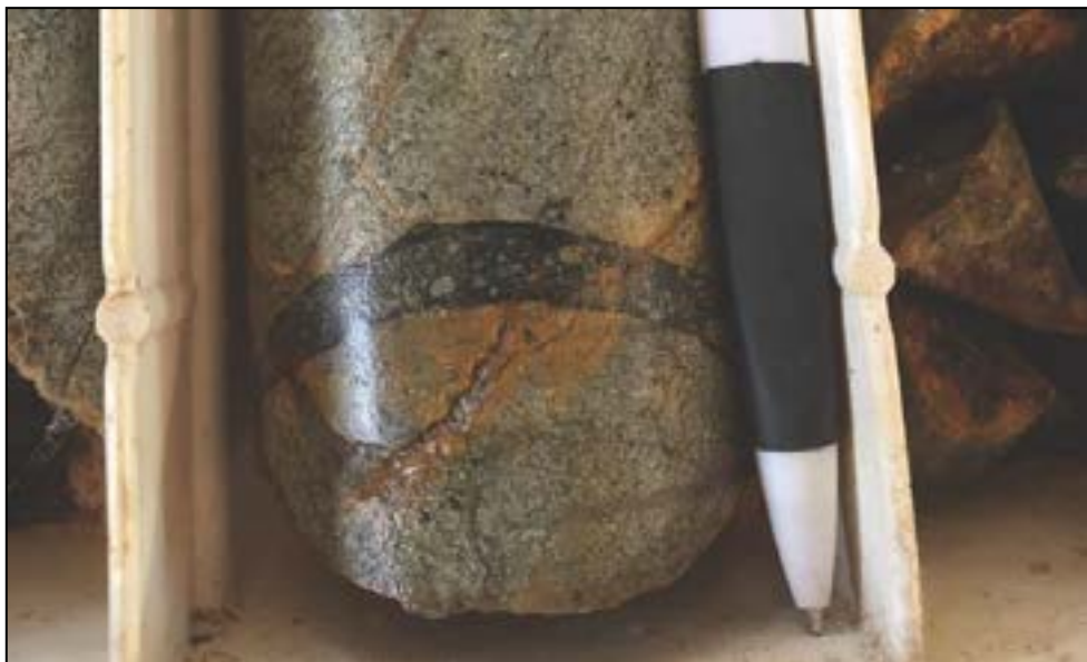
Figure 3-65: Band of mylonite in drill hole F4 that offsets partially oxidised fractures/ joints
