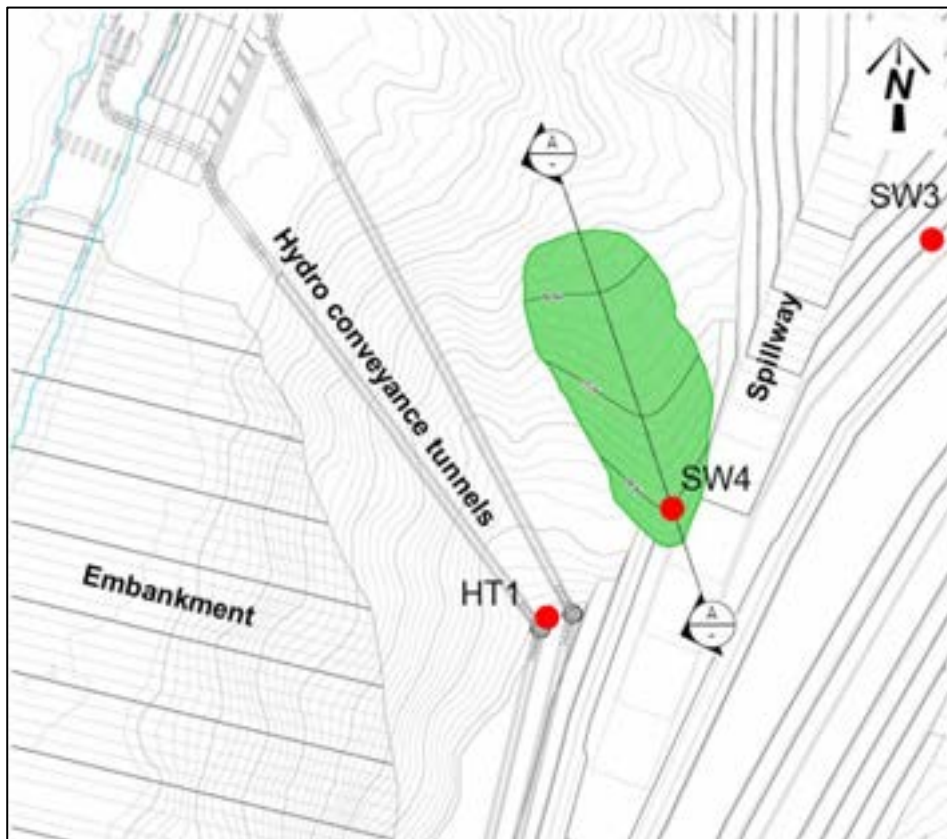
Figure 11-7: Plan view of potential unstable zone (in green) and drillhole locations in the right abutment
