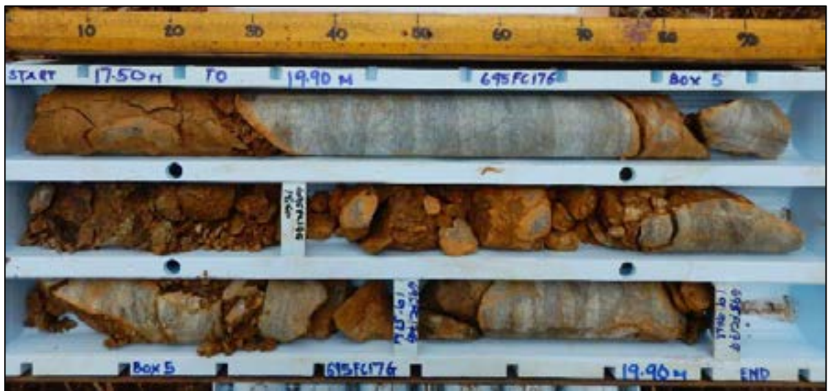
Figure 11-9: Drillhole SW4 from 17.5 to 19.9 m, showing boulder overburden material over the bedrock
