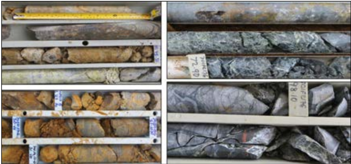
Figure 3-96: Examples of poor quality drill core from the southern part of the quarry
