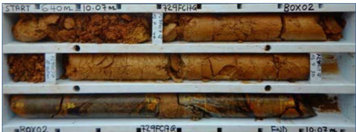
Figure 11-11: Core photograph showing soil-like overburden material immediately above highly fractured rock in drillhole LH7, from 6.4 m to 10 m depth
