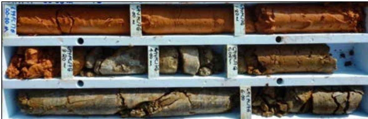
Figure 3-21: 3 m of soil-like colluvium in drill hole SW5
