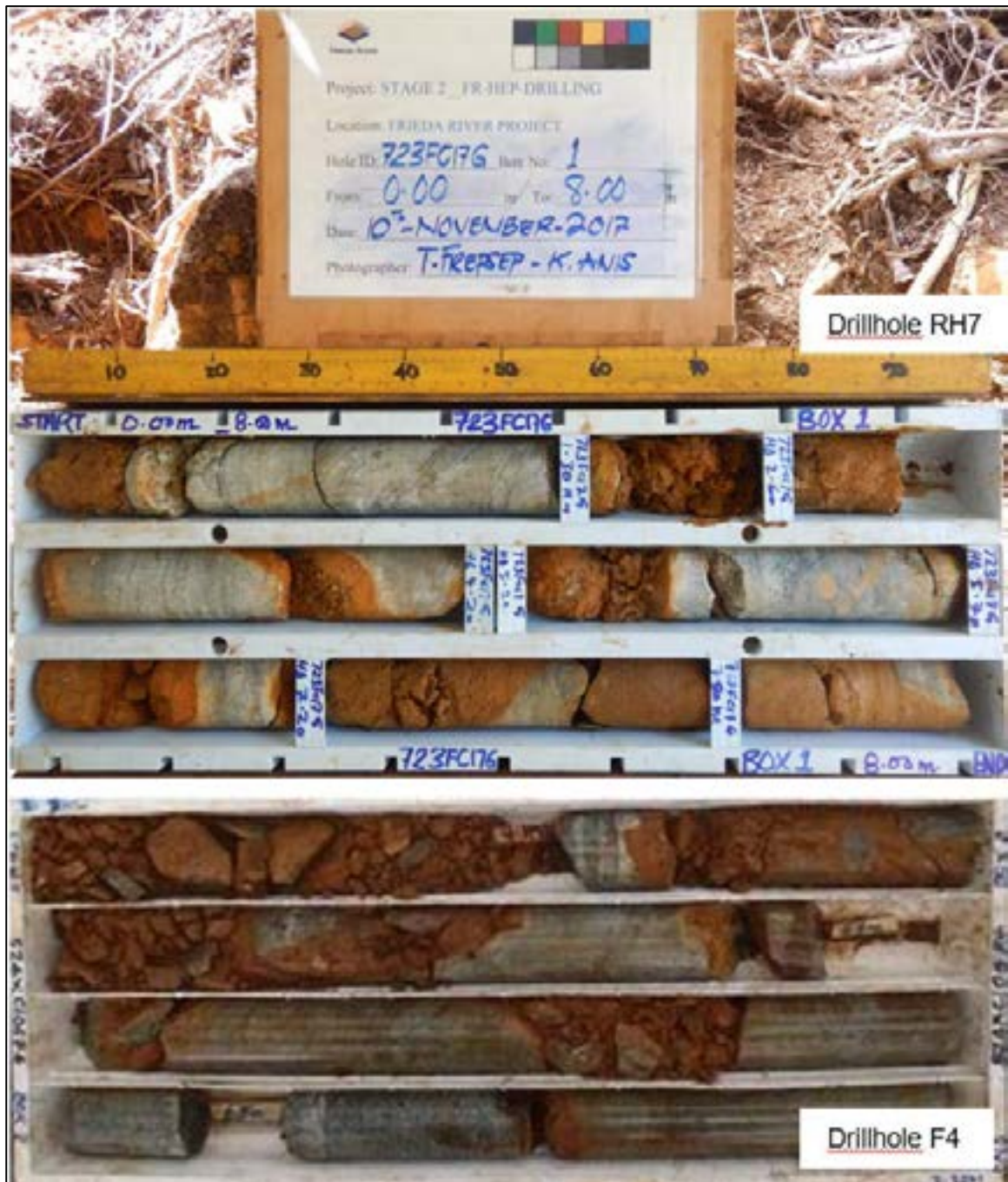
Figure 8-4: Core photos from holes RH7 and F4 – the Frieda River riverbed representative of foundation level (~5 m)
