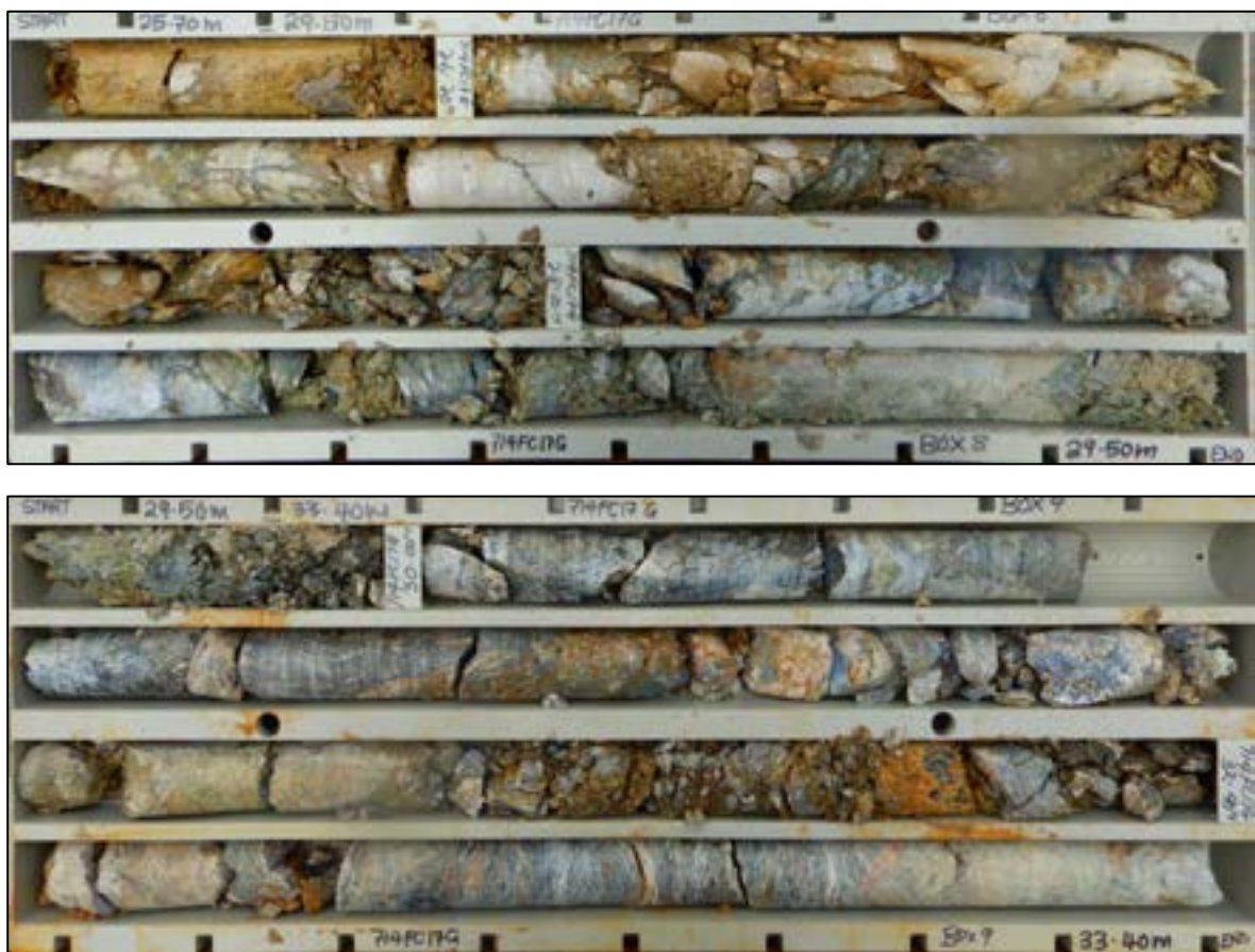
Figure 3-36: An example of third order fault conditions – highly fractured and sheared rock
