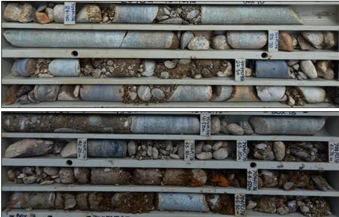
Figure 8-10: Typical core from the Frieda River valley floor showing uncemented (2b) material
