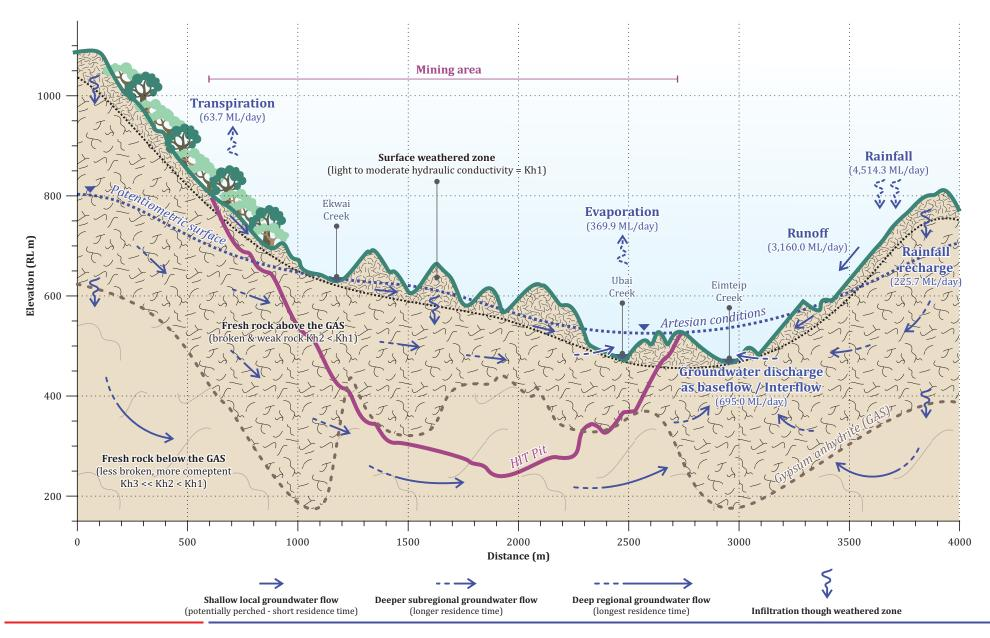
Schematic section of conceptual hydrogeology - HIT open-pit
