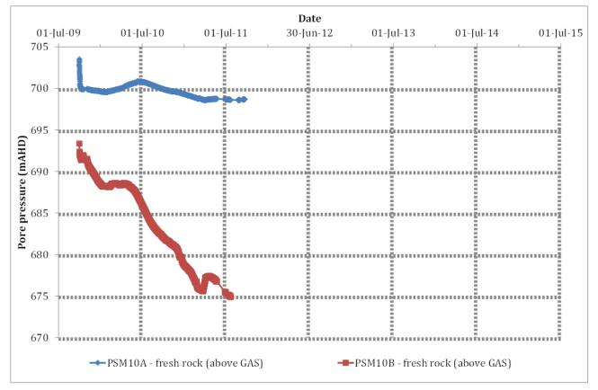
Figure 4.8 VWP hydrograph - PSM10
