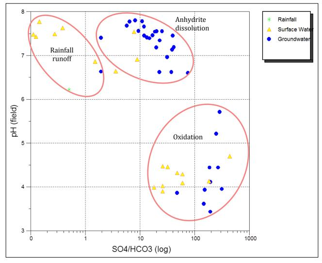
Figure C 3.5 Scatter plot SO<sub>4</sub>/HCO<sub>3</sub> versus pH
