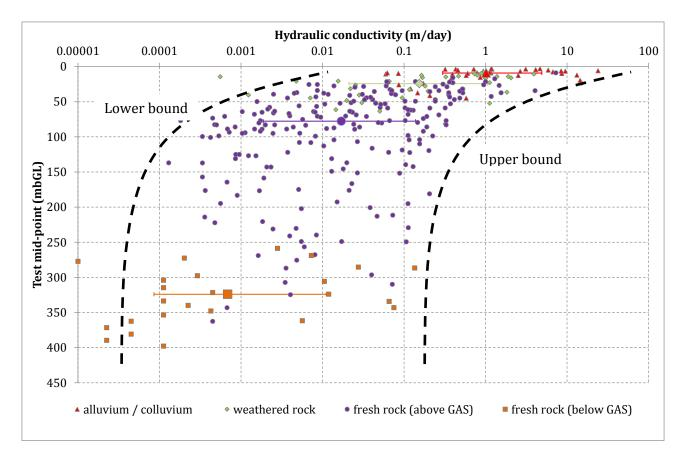
Figure 4.9 Hydraulic conductivity with depth
