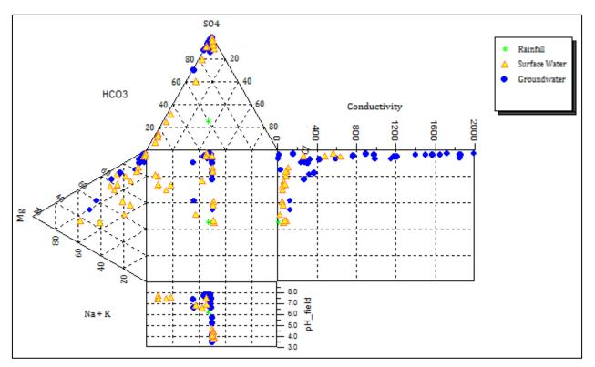
Figure C 3.3 Durov plot of water sample chemistry
