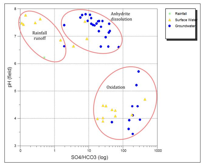
Figure 4.15 SO<sub>4</sub>/HCO<sub>3</sub> versus pH
