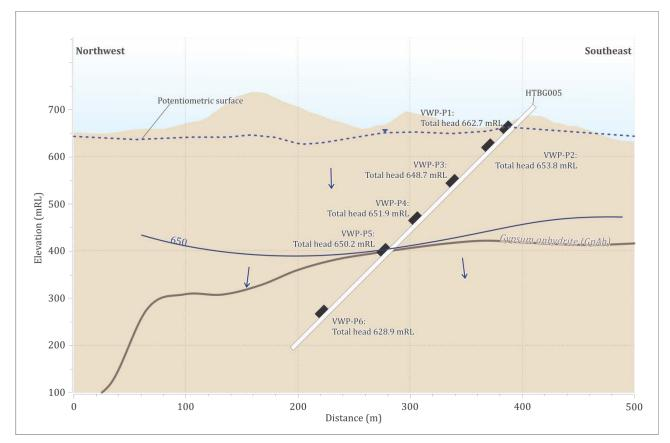
*Note:* blue lines represent lines of equal head, the arrow indicate flow direction
