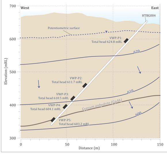
*Note:* blue lines represent lines of equal head, the arrow indicate flow direction
