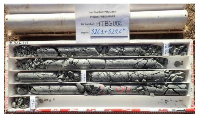
Figure 4.10 Example of broken core above the GAS
