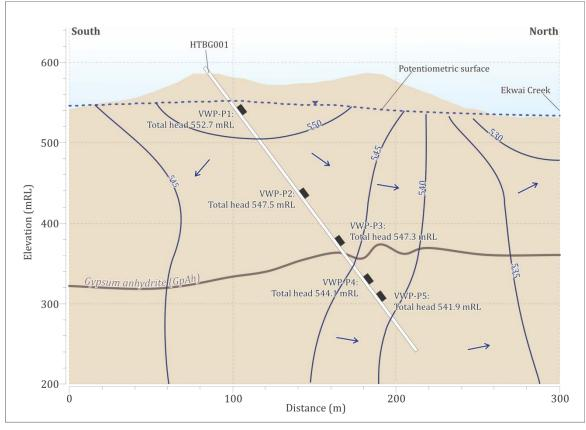
*Note:* blue lines represent lines of equal head, the arrow indicate flow direction
