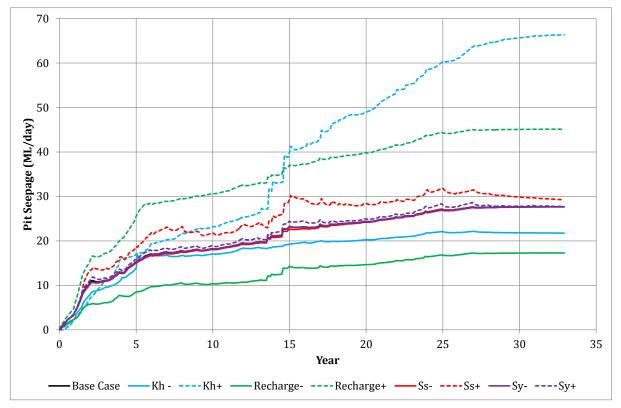
Figure 6.7 Sensitivity – Predicted open-pit groundwater seepage
