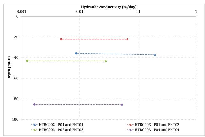
Note: circles represent packer test data and triangles represent falling head data
