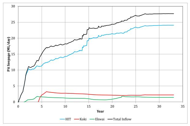
Figure 6.3 Predicted groundwater open-pit seepage
