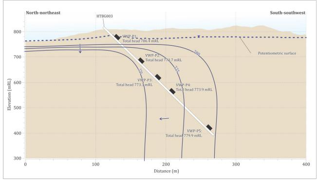
*Note:* blue lines represent lines of equal head, the arrow indicate flow direction
