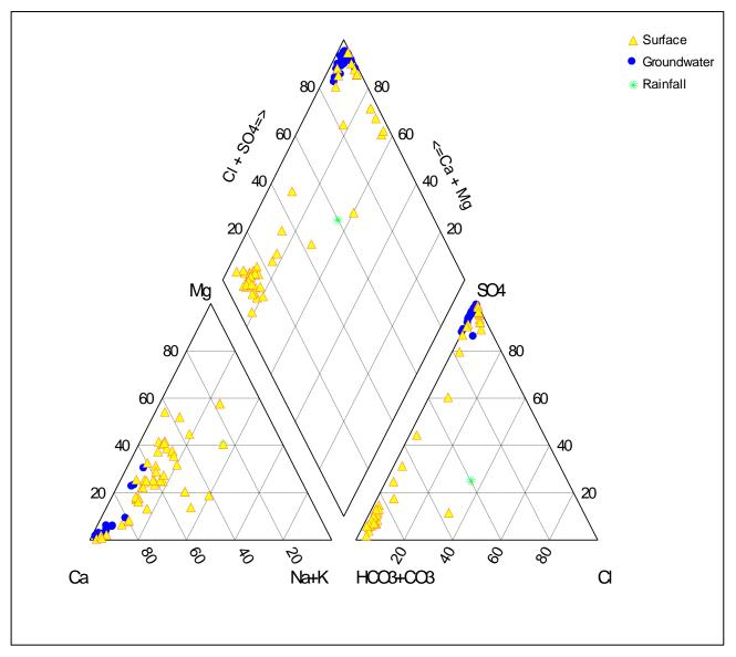
Figure C 3.4 suggests that major ion ratios are similar for all artesian exploration drill holes with samples plotting in a similar section of the piper diagram (dominated by Ca and SO<sub>4</sub>).
