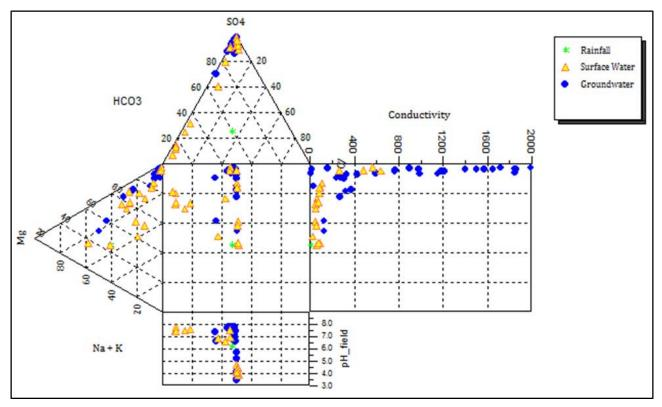
Figure 4.14 Durov diagram
